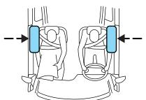
• Two crash sensors located under the outboard side of the front seats, attached near the floor.
